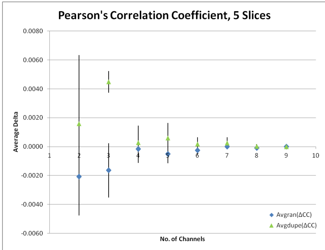
Figure 24: Monte Carlo Simulation PCC 5 Slices. Each data point represents the average delta from adding a random or duplicate channel. The graph shows that the average delta is less when a duplicate channel is added to the data.
