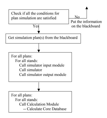
Figure 5: The procedure for plan simulation
