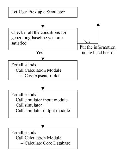
Figure 4: The procedure for baseline generation
