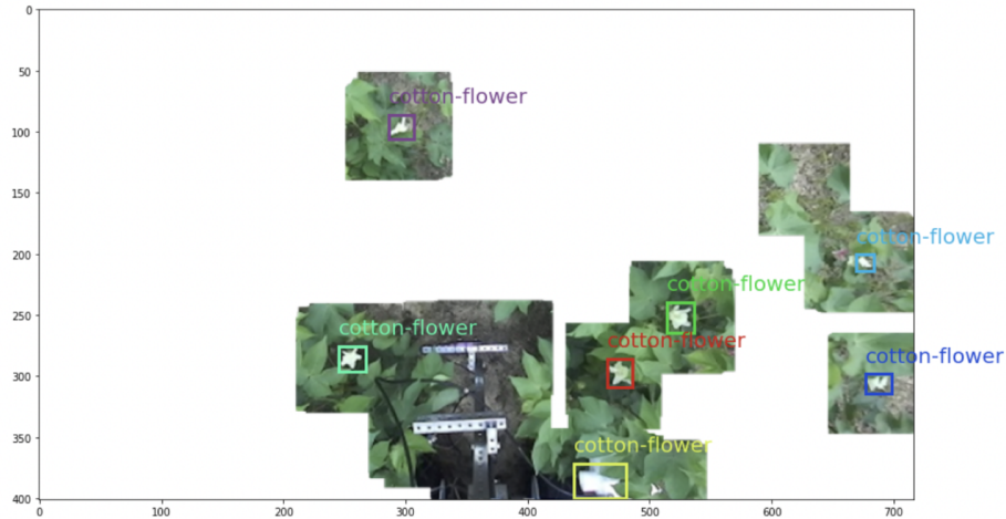
Figure 4.15: An example of pipeline output on 2022 Data with Masking and Downsampling, Preserving 50 Non-White Regions around Binary Classified White Region.
