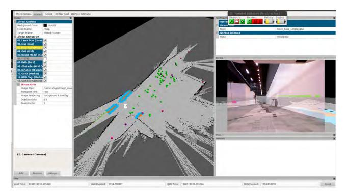
Figure 1.5: RVIZ During one of A.T.I.C.U.S.S.'s runs. The Green Dots are RFID tags. On the right is a feed from the Kinect Camera onboard.
