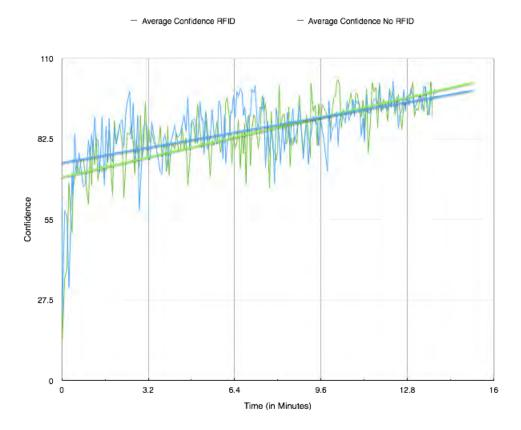
Figure 4.13: Average Confidence over Time, Green being without RFID tags, Blue with RFID  $% \left( {{\mathbf{F}_{\mathrm{S}}}} \right)$
