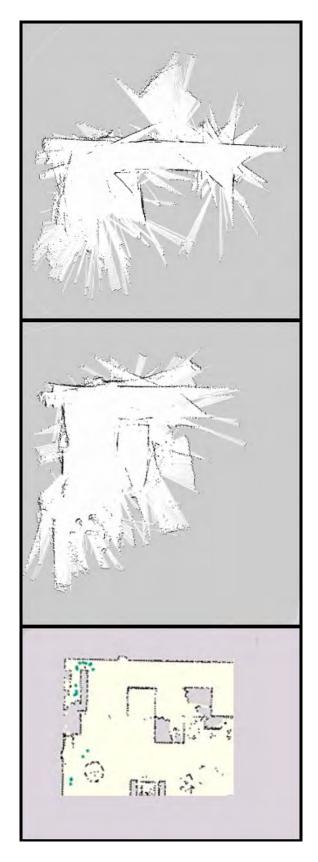
Figure 5.2: Comparison of different methods. From top to bottom: Greedy with RFID turned off, Greedy with RFID turned on, and the SRI Developed Map, zoomed in.
