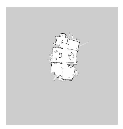
Figure 4.11: Map of A-smart-ment made using RFID tags
