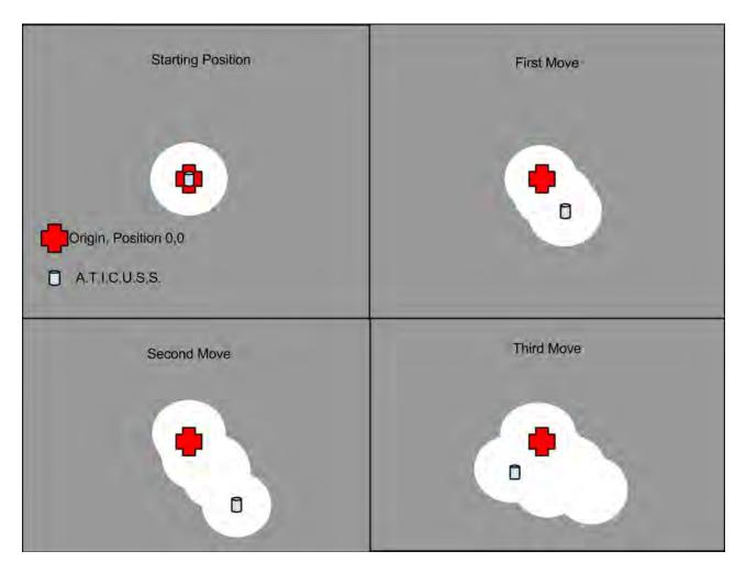
Figure 3.2: Explanation of Exploration: white is the known map, grey is unexplored space. At the end of the third move, the robot's current map is larger than the start. It can now move to any area in white and further expand the map.
