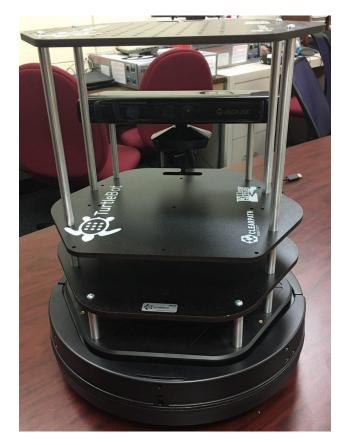
Figure 5.7: This is the Turtlebot that has been used on our experiment. Each Turtlebot is equipped with a Microsoft XBox 360 Kinect, which provides a camera, a ranging sensor, and a microphone.
