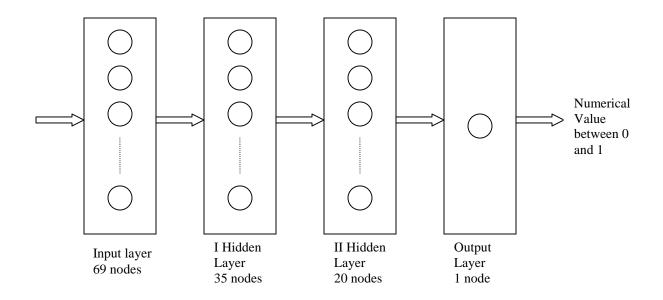
Figure 2. 1 Back Propagation Artificial Neural Network for Three-state classification system for Fort Valley for a prediction period of twelve hours.
