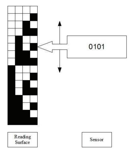
Figure 1.1 - An example of a linear encoder in action. As the sensor moves vertically, in relation to the reading surface, the pattern changes, and so does the resulting binary interpretation.
