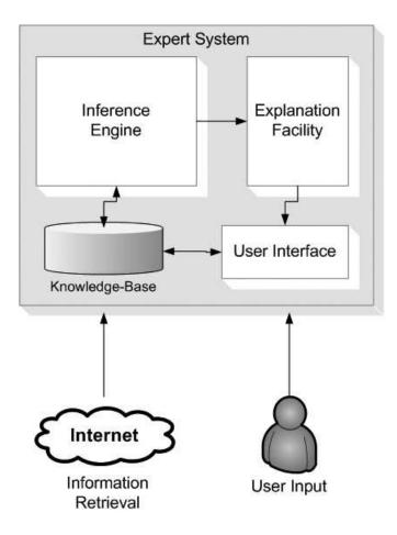
Figure 2.3: Expert System module
