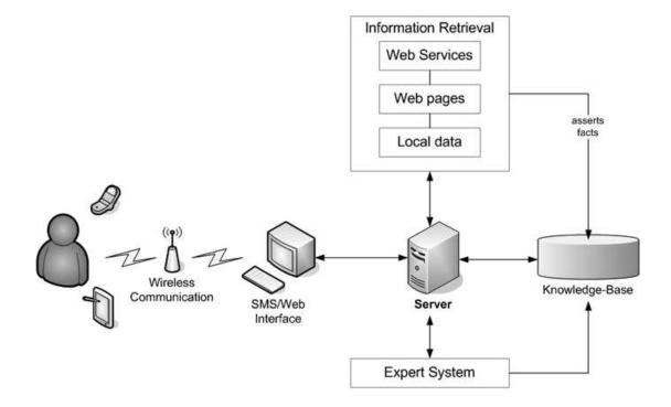
Figure 2.1: System architecture
