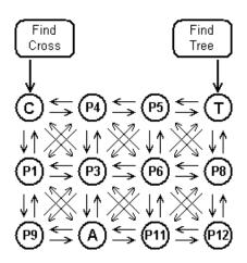
Figure 8: Tree and crossfinding goal behaviors (T & C) activate position behaviors, which spread activation toward the agent (A) through move behaviors
