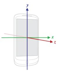
Figure 2.1: Android sensor coordinate system<sup>1</sup>
