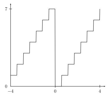
Figure 2.1: The staircase wave discretization function
