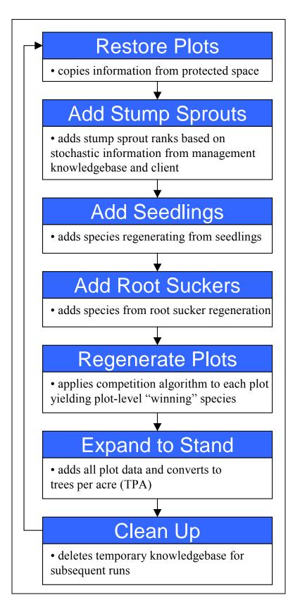
Figure 3.4: Core Engine Regenerate Stand Flow
