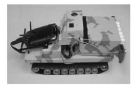
Figure 3.6 The Modified Tank Chassis
